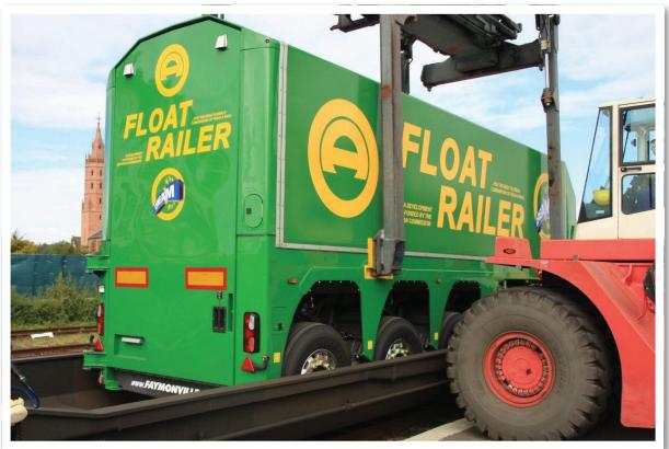
Figure 6-6: Intermodal semi-trailer for plate glass transport
