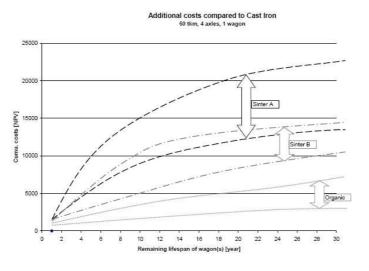
Figure: Influence of LL-blocks on LCC. [Source The Whispering Train Programme - Life Cycle Cost calculation – Intermediate Report – Lloyd's Register]
