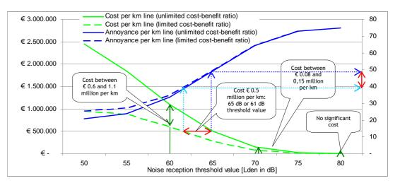
Figure 23: Cost for noise control and annoyance for different threshold values per km railway line.
