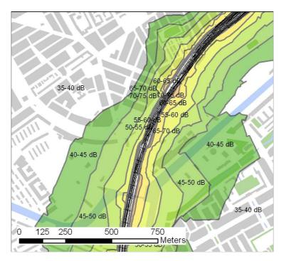
Figure 18: Example of distance of railway noise levels for present situation (L<sub>night</sub>).
