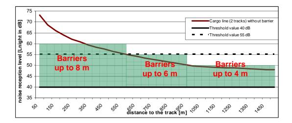
Figure 30: To reduce noise reception levels to 40 dB ( $L_{\text{night}})$  requires high barriers up to large distance of the track for cargo lines.
