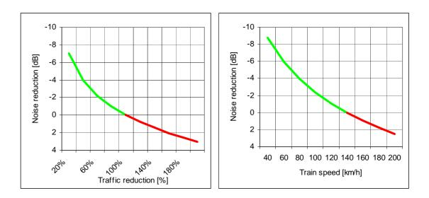
Figure 35: Substantially operational measures like traffic reduction and reduction of train speed do have a relative small impact noise reduction.
