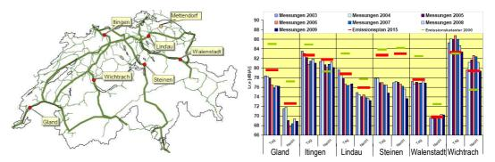
Figure 13: Swiss monitoring of actual emission level, compared to Emission Plan 2015 (----). Source: www.bav.admin.ch.
