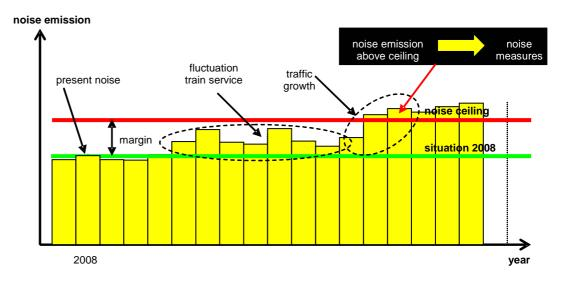
Figure 21: Graphical presentation of the 'Dutch system' of noise emission ceilings. The margin is 1.5 dB on the whole network.
