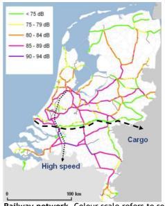
**Railway network.** Colour scale refers to socalled 'Noise creation value', as defined in Dutch calculation scheme
