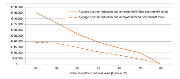
Figure 24: Average cost for noise reduction of one annoyed person for different threshold values relative to a threshold value of 80 dB.
