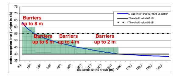
Figure 31: To reduce noise reception levels to 40 dB  $(L_{\text{night}})$  requires high up to large distance of the track for mixed lines.
