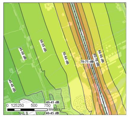
Figure 33: Example of distance of railway noise levels ( $L_{night}$ ) for present situation. The number of trains used in this figure does not match the number of trains in Figure 25.
