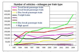
Still a considerable number of passenger trains with cast-iron blocks (type 1 and 2) is running on the Dutch network.
