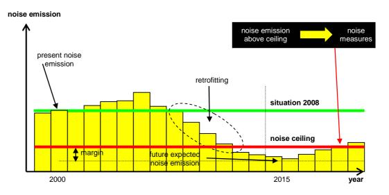
Figure 22: Graphical presentation of the 'Swiss system' of noise emission ceilings. The margin is different for different railway lines, based on a traffic prognosis for each line.
